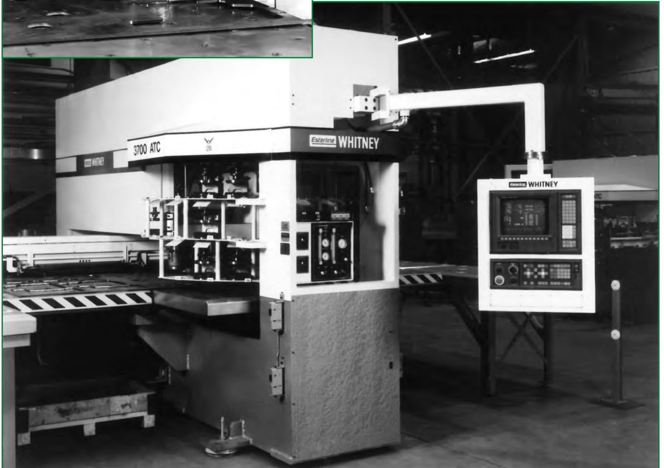
Punch/Plasma Fabricating Center combines punching/cutting into a single operation.
