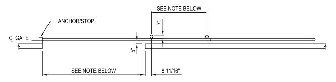
NOTE: DISTANCE FOR OVERHANG POSTS IS 66% MIN. OF OPENING
